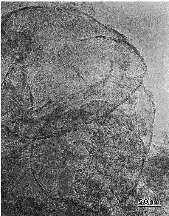
Fig. 5 High resolution TEM image of balloon-shaped particles contained in the shock-compacted sample.
